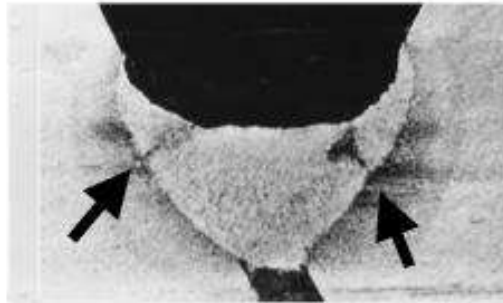
Sulfur crack in SMAW
